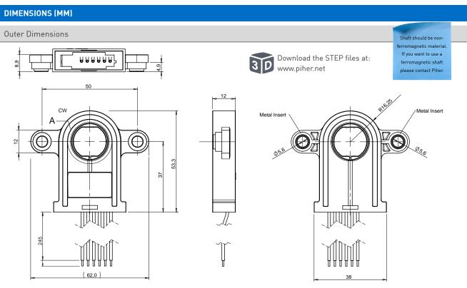
Sensor shown above is the 17mm version with the rotor at zero position. Sensor is delivered at random position. Wires: 0.35mm² TXL SAE J1128
