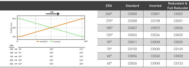
All output functions listed are centered in 180°. Output level from 10% to 90%
