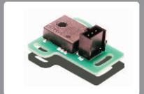
The MTS-360PCB Sensor/PCB assembly is available with either 6 pin (dual output) or 3 pin (single output) Molex 90119 Series mating connectors. The PCB / Sensor assembly can be easily secured with three standard M3 screws. The entire assembly measures just 35mm wide by 36mm long and 7.5mm high, allowing for applications with tight packaging constraints.
