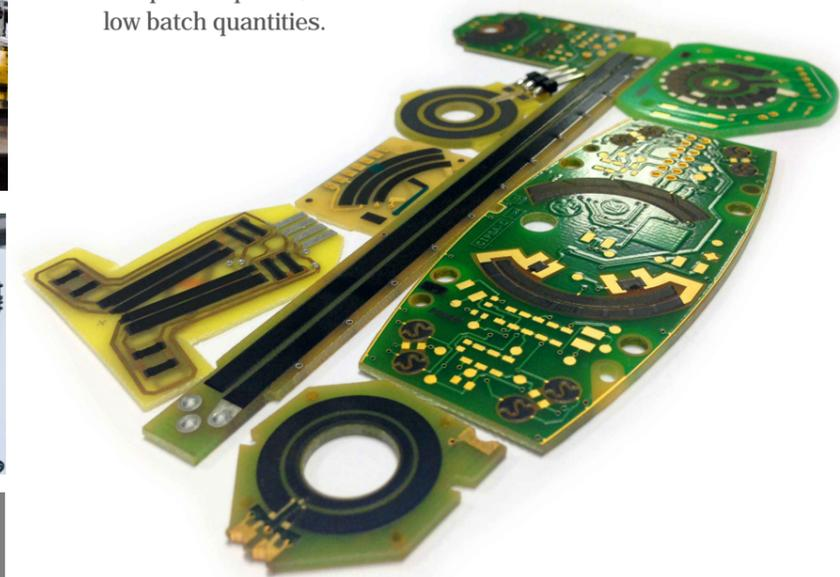
Once screened and cured, these resistive tracks can be individually laser trimmed to obtain very accurate tolerances in high volume.
