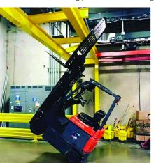
To provide additional safety, the speed of the vehicle can be limited, based on the height of the mast, reducing the possibility of a vehicle tipping over.
